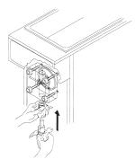
Figure Q Installing Plunger and Spring
